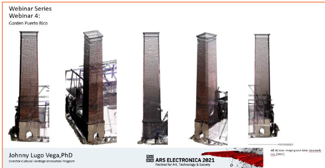
Figure 9. Example of 3D scan of Hacienda Mattei's Sugar mill as a new technology approach in sustainable conservation.
